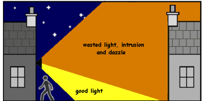
Figure 1: poor positioning and poor direction
