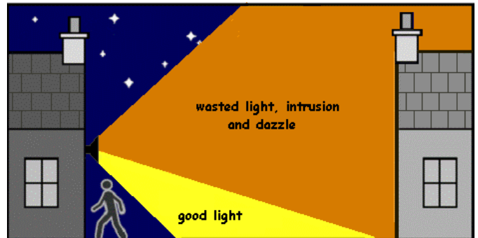
Figure 1: poor positioning and poor direction
