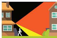
Figure 1: poor positioning and poor direction
